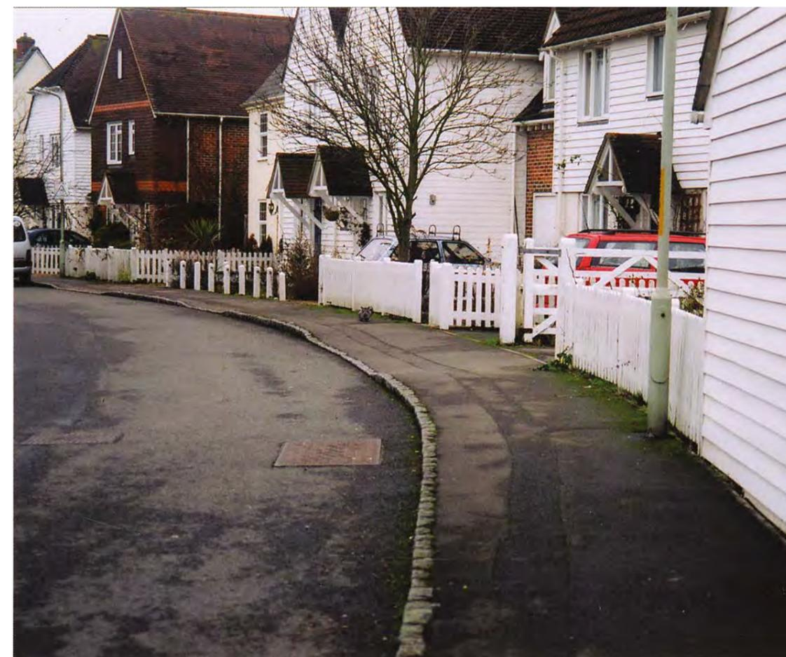
Figure 192: Blacktop carriageway and footway with small element kerb
