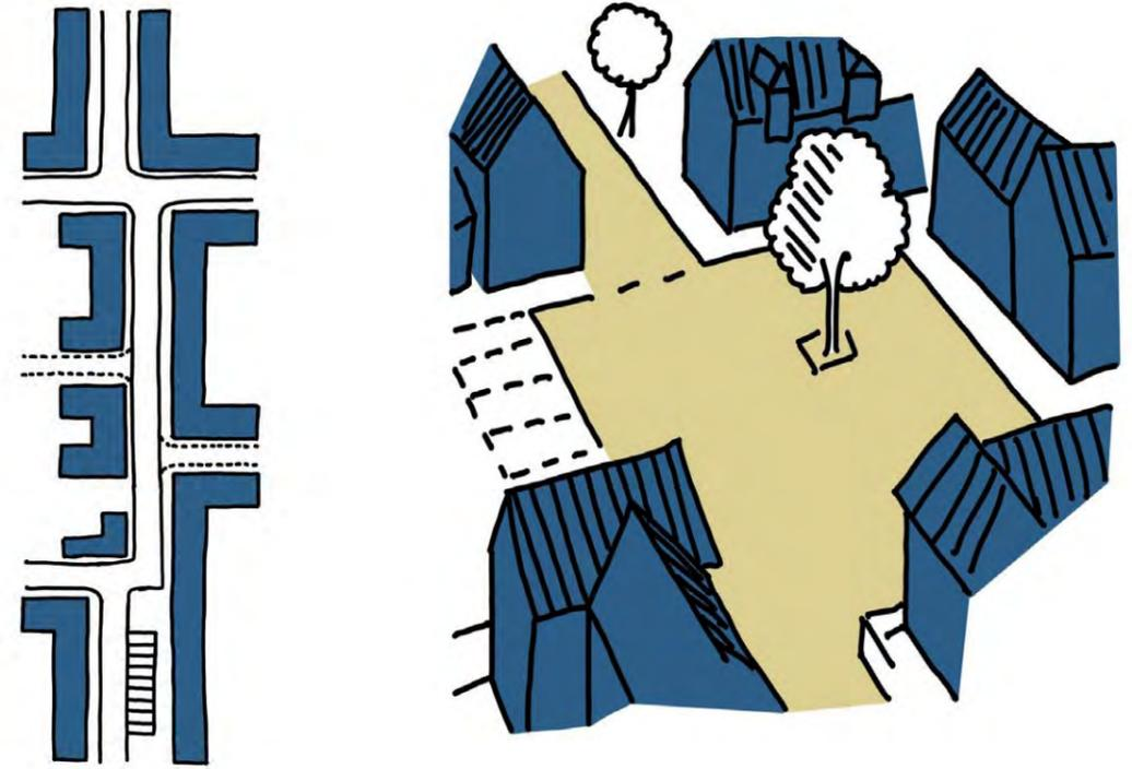
Figure 176: (left) Frequent changes of direction and tight corners with narrow sight lines can, where appropriate, control speed (these should be checked by tracking and compliance with the appropriate standards)
